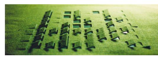
typology: the roof structure and form refers to the sawtooth roofs of industrial constructions: the building boasts constant light levels, due to the bulk of light arriving by the north facing glazed wall, as well as a constant daytime temperature due to the integrated system of natural ventilation and the insulated roof which reduces direct solar gain.
