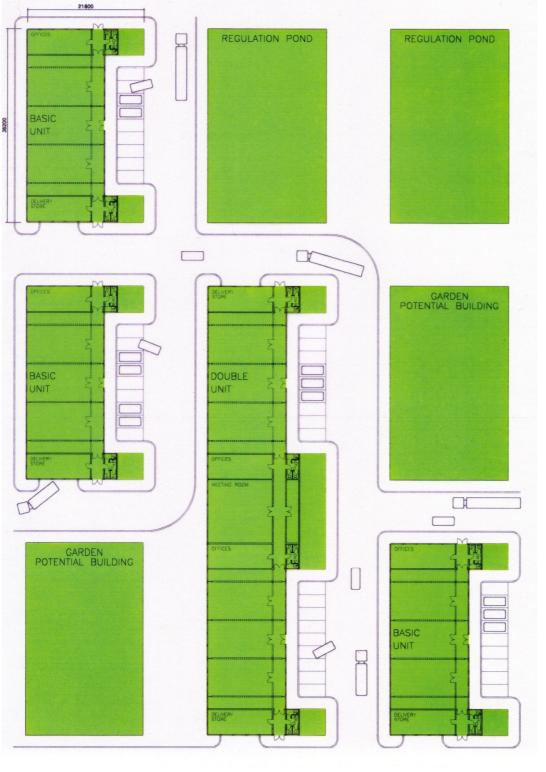
unitary flexibility: the building type is capable of both being divided into smaller units or being joined with its neighbour. to enlarge the working surface without reducing the green area, the buildings have the potential include to system mezzanines. this offers the possibility of many different functional variations based on the same diagram.
